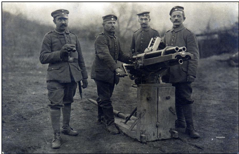
Figure 6: 37 mm Gruson-Hotchkiss Revolverkanone revolving-barrel anti-aircraft gun that fired the strings of ‘flaming green onions’ reported by the night bomber Handley Page O type crews (courtesy of the Brett Butterworth collection)
