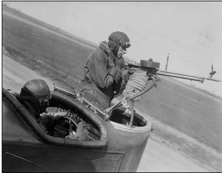
Figure 4: The observer and pilot in a Handley Page O/400: Observer in the nose cockpit, manning a single Lewis gun mounted on a Scarff ring near Cressy, 25 September 1918: Photograph by 2/Lieutenant David McLellan (Public Domain - United Kingdom Government and taken prior to 1 June 1957)
